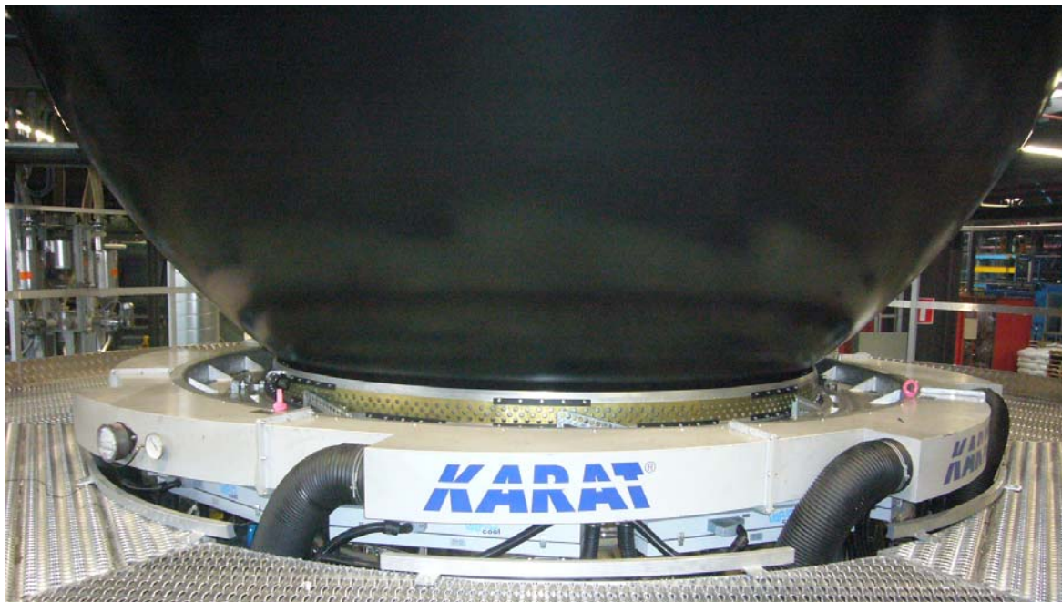
Air ring KARAT for die 2000mm with motor-driven lip adjustment and gauge control system VARIOcool (picture 2)
